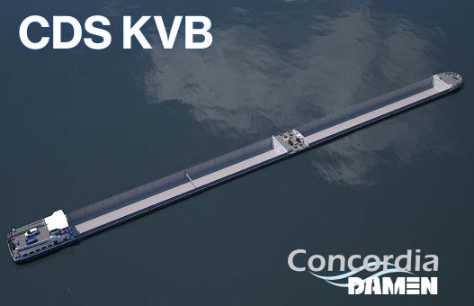
Concordia Damen's 'CDS KVB' ('koppelverband') combination vessel allows skippers to sail longer at low tides and shallow water levels, a useful feat in the current climate.
