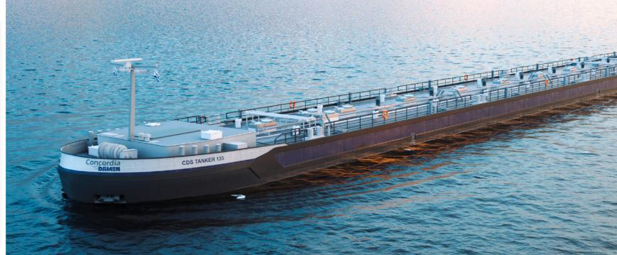
The fuel-efficient CDS 135 Tanker has minimal resistance and an optimal 'speed-power curve'. The innovative design allows for smaller propellers, which is very useful when water levels are low.
